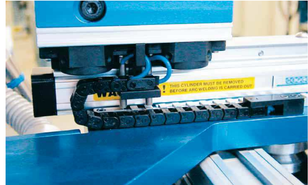
Series 03 - extremely small installation space on a paint-spraying machine
