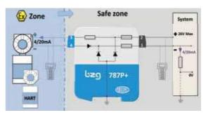
A Zener barrier is designed to limit energy that may appear in hazardous area whatever the type of connection made before the barrier.
