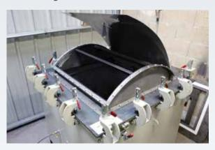
We test the vent panels in our factory according to EN 14797. These panels are manufactured under the CE examination certificate type INERIS 15ATEX0038X and the quality managment system of the company is certified by the CE quality certification FSA 15ATEXQS019.
