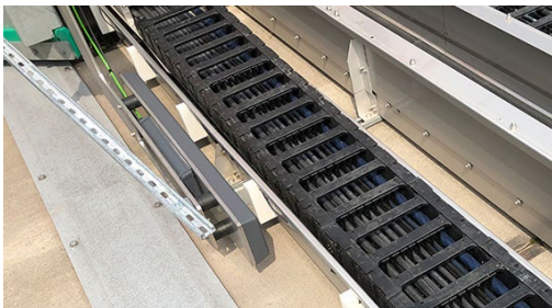
P4.1 e-chain® with EC.PP in the igus® outdoor test (left) and control cabinet with smart plastics modules (right)
