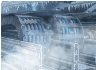
Climate chamber: dynamic tests of cables in e-chains® at -40°C
