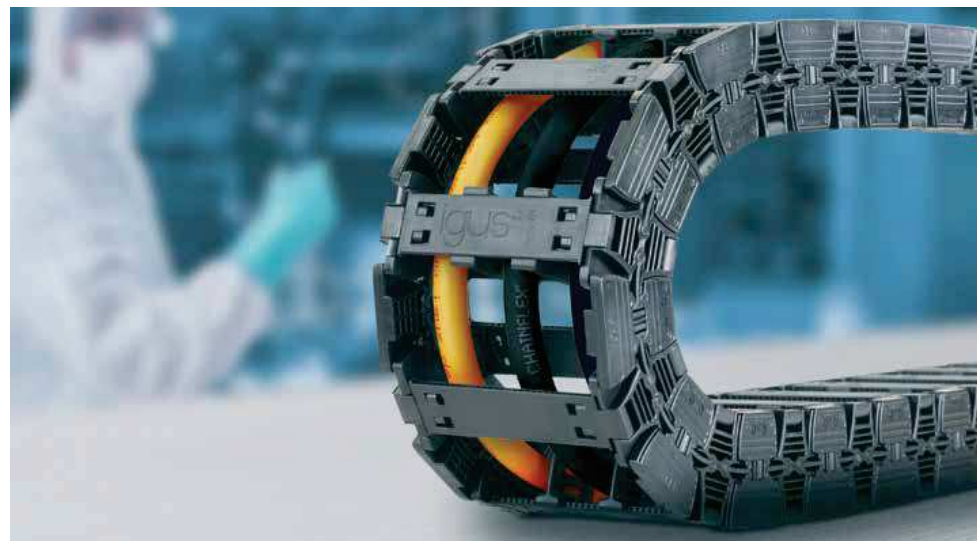
The interior of the E6.1 has been designed to be extremely cable-friendly to increase the service life of cables and hoses even more. The crossbars are very smooth and rounded as is the transition from e-chain® link to crossbar, and all markings have been moved outside of the e-chain® cross section.
